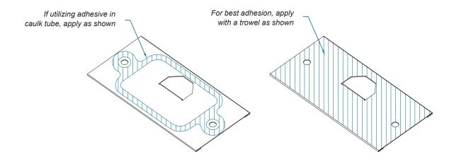
Place the DABs into the locations defined on previous page, under Installation. Firmly press down to distribute the glue and install the spiral anchors through the two holes located near the edges of the bracket.
