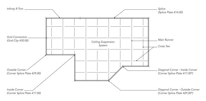
\* Field modify Corner Splice Plate to achieve desired angle greater than or less than 90°.
