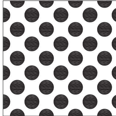
K 250R354D 0.25" Diameter holes 0.354" Diagonal centers 39% Open area
