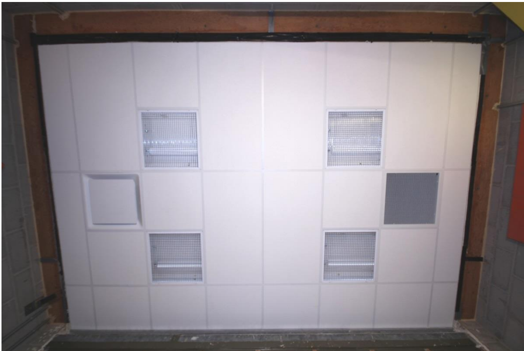
Fig. 3 – The typical ceiling system configuration used throughout the testing with various acoustic ceiling panels suspended in a metal grid and with light fixtures and supply and return air devices.
