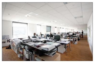
Stone wool ceiling panels may be specified for their light reflection to extend the sunlight more deeply into the workspace, which helps reduce the need for electrically powered lights (and the associated energy costs).
