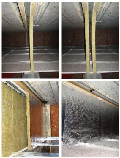
Figure 10: Lightweight, stone wool, plenum barriers installed above the central demising wall of the laboratory's chamber during testing. Top-left: Single-layer. Top-right: Double-layer with a 1-5/8 inches airspace in between. Bottom-left: Double-layer with seams staggered and small cuts at the bottom so the panels slide down over the grid bulb. Bottom-right: Installation complete with tops screwed, seams taped and ceiling panels installed.
