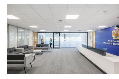
These elegant, frameless acoustic islands are suspended in a linear formation by wires affixed to the three metre high plenum but they can also be installed using a suspended grid or fixed directly to the soffit. They absorb sound on both sides, helping to reduce reverberation time and improve ambient sound levels. Their smooth, deep matt, super white surface has anti-static properties which extend product life.
