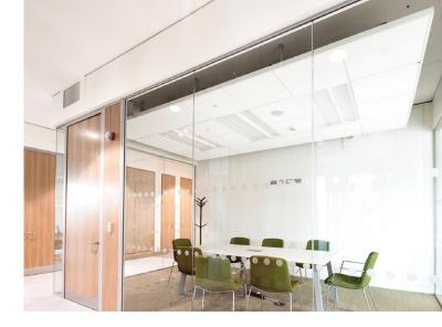
light reflection and light diffusion to create a bright and comfortable environment that helps meet the university's brief for well-lit spaces. The islands are constructed to provide high sound absorption and sound insulation, ensuring conversations inside the rooms remain private and undisturbed by external noise.
