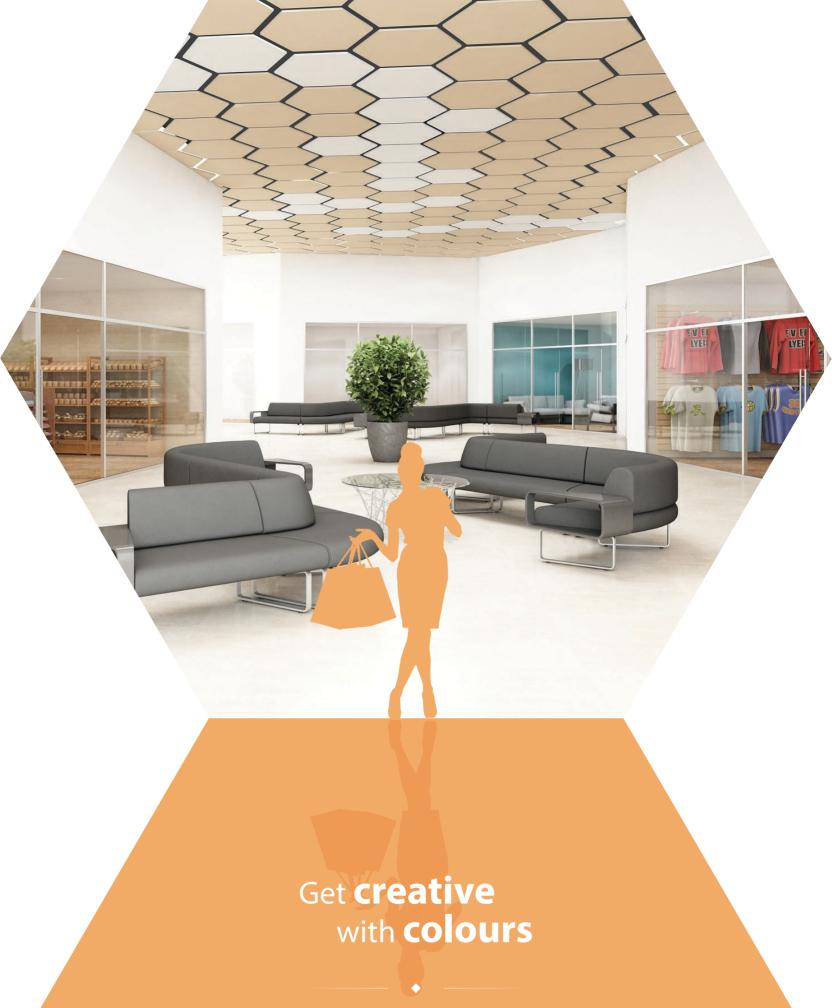
Rockfon Eclipse is available in white and and in an unlimited number of custom colours. Each island is made of a 40mm-thick stone wool panel. The visible side is covered with a painted glass fleece that creates a smooth surface. The rear side can be ordered in the same colour as the front side, or in white to enhance light reflection.
