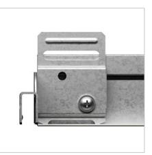
Bridging bracket for T profiles to your main runners and cross tees, transferring the weight of the service to the grid. This ensures that no load rests on the tile, eliminating concerns of deflection.
