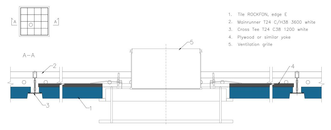
This solution is applicable for grilles (services) weighing <3kg.
