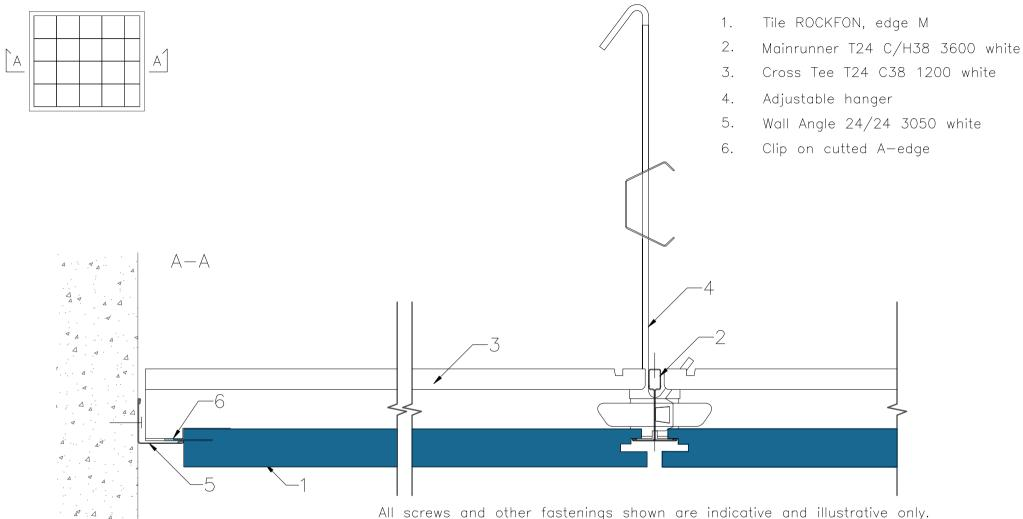
Specific fasteners should be chosen dependent on substrates and materials being used.
