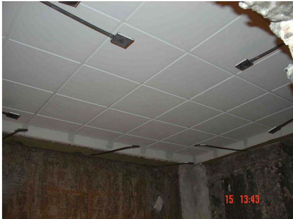
Figure C1 Specimen from the heated side before the test
