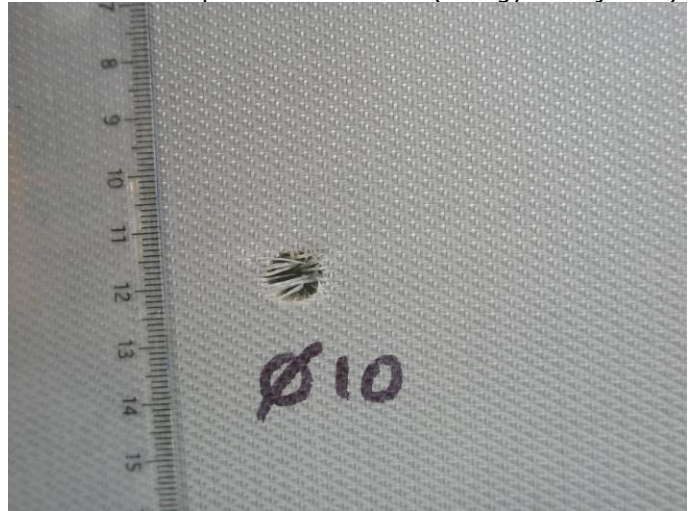
Partial puncture examination \varnothing 12 mm (energy 3.75 joules)
