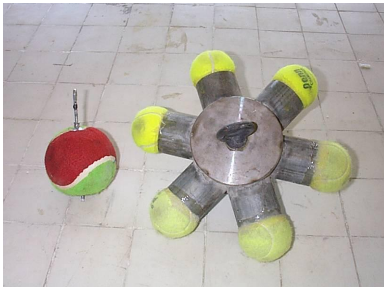
Photograph no. 4: Test apparatus – tests of impacts with ballasted tennis ball and special ball
