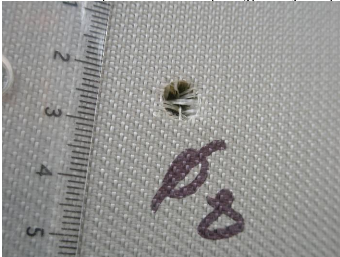
Partial puncture examination \varnothing 12 mm (energy 3.75 joules)
