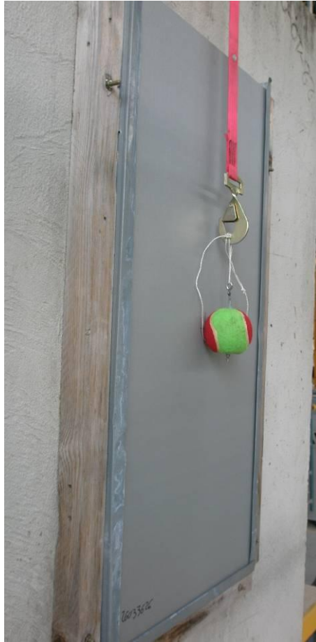
Photographs no. 1 to 3: Apparatuses of tests – Impacts from tennis ball, special ball and football
