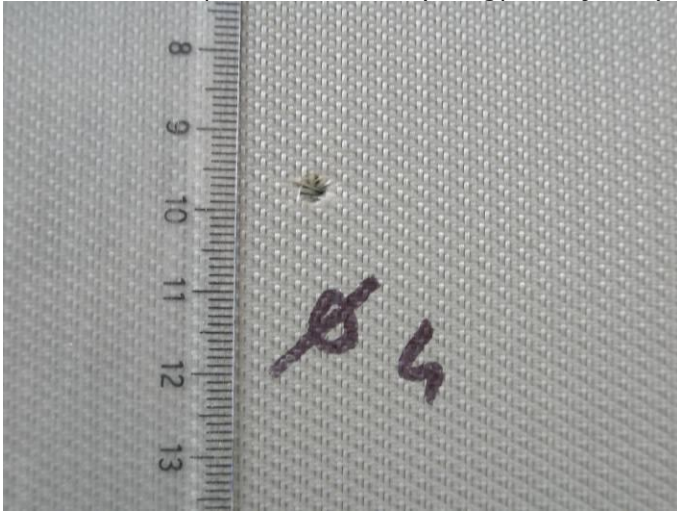
Examination of puncture \varnothing 8 mm (energy 3.75 joules)
