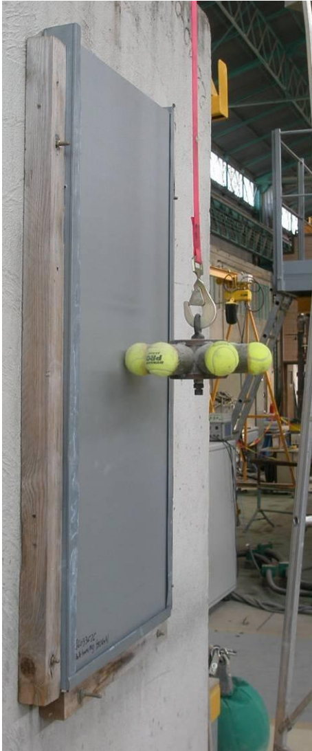
Photographs no. 1 to 3: Apparatuses of tests – Impacts from tennis ball, special ball and football
