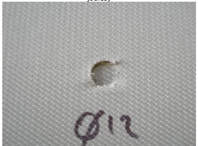
Partial puncture examination \varnothing 12 mm (energy 3.75 joules)
