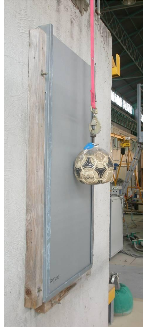
Photographs no. 1 to 3: Apparatuses of tests – Impacts from tennis ball, special ball and football
