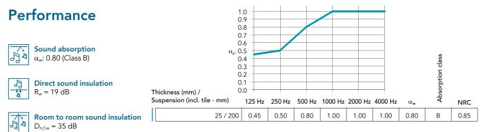
The sound insulation properties (R<sub>w</sub>, D<sub>n,f,w</sub>) presented
