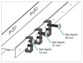
Make sure to select the screw that matches the deepest slat used in the specific installation.
