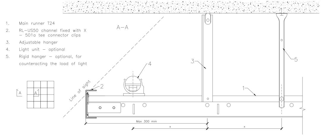
Floating ceiling incorporating optional light and counteracting rigid hanger. For the best aesthetics, hangers shall be positioned so that they are not seen from floor level, and the surrounding RL-US50 (or deeper) channels shall be fixed using X-501a tee connector clips, thereby avoiding visible fixings.
