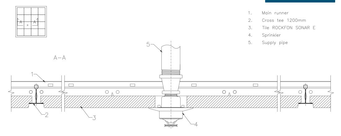
Cut hole in tile and attach sprinkler head to supply pipe.
