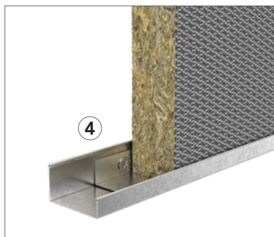
The 40 mm J-channel (25/40/13 mm) and the supporting bracket to support the bottom of the panels mounted at multiple heights or off the floor.
