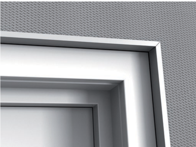
3.9 J-channel finishing around a door or window should always be done with J-channel mounted with a 25 mm wide-edge to the wall, affixed every 300 mm and 30 mm from all ends. To minimize panel waste, measure and cut carefully while ensuring adequate J-channel overlap.
