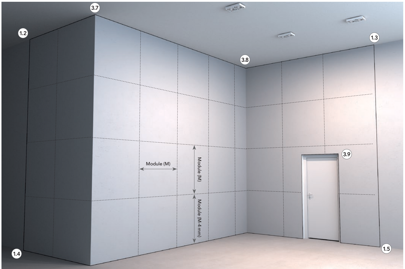
1.1 Mark out all the axes for J-channels and intermediate profiles at Module (M) measures. For the bottom row of panels, use M-4 mm up from the bottom J-channel.
