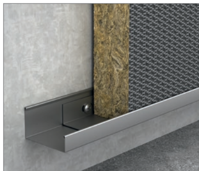
40 mm J-channel (25/40/13 mm) and the supporting bracket are used to support the bottom of the wall panels when mounted at multiple-heights or off the floor. When using the 1 mm thick J-channel, supporting brackets are not needed.
