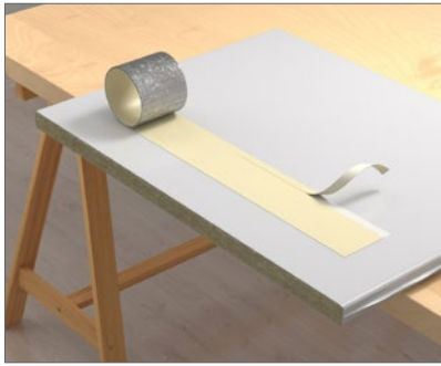
2. Measure edge + 10 mm and peel.
