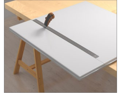
1. Cut to required dimensions.
