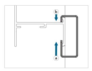
a) First insert the bottom part of the Universal Bracket onto the Middle profile and push it up.
