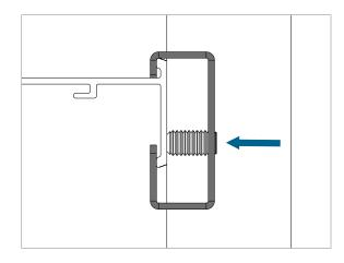
Fasten the set screw to secure the Universal Bracket onto the Middle profile.
