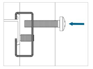
Insert the suspension screw in the Universal Bracket.
