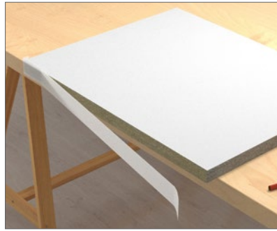
3. Align 5 mm overlap on front and press.
