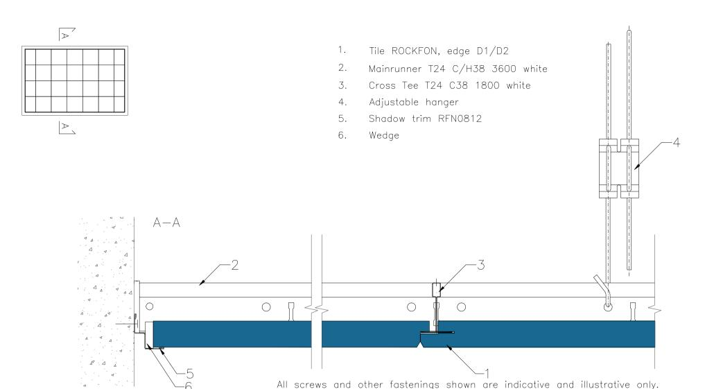
Specific fasteners should be chosen dependent on substrates and materials being used.
