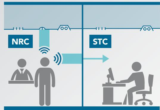
Comply with sound blocking requirements between rooms (STC) with full-height walls. Comply with sound absorption requirements within rooms (NRC) with high performance Rockfon stone wool ceiling panels.
