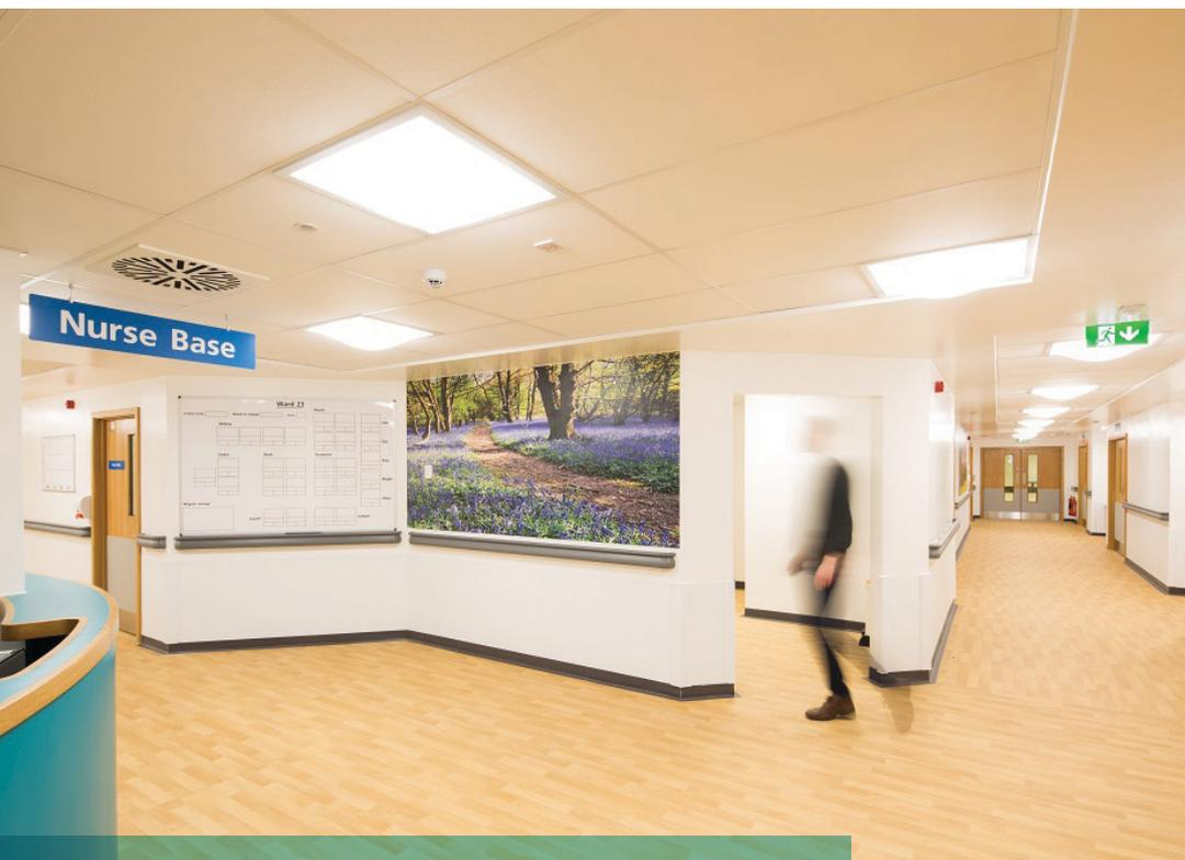
Rockfon MediCare Air benefits from having a high-performance membrane and sealed edges. Combined with MediCare clips, the ceiling can achieve an air leakage rate of less than 0.5m<sup>3</sup>/h/m<sup>2</sup>/Pa under a pressure range of 5 to 40 Pa. Rockfon MediCare Air also offers the highest safety (Class A1), excellent sound absorption (Class B).
